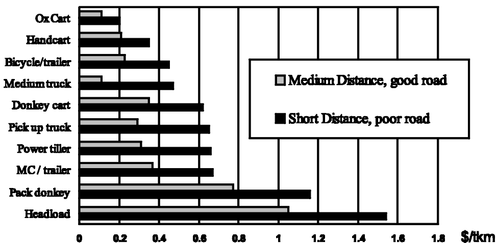
Figure 1. Transport costs for different vehicles in developing countries (data from Crossley and Ellis 1997).
